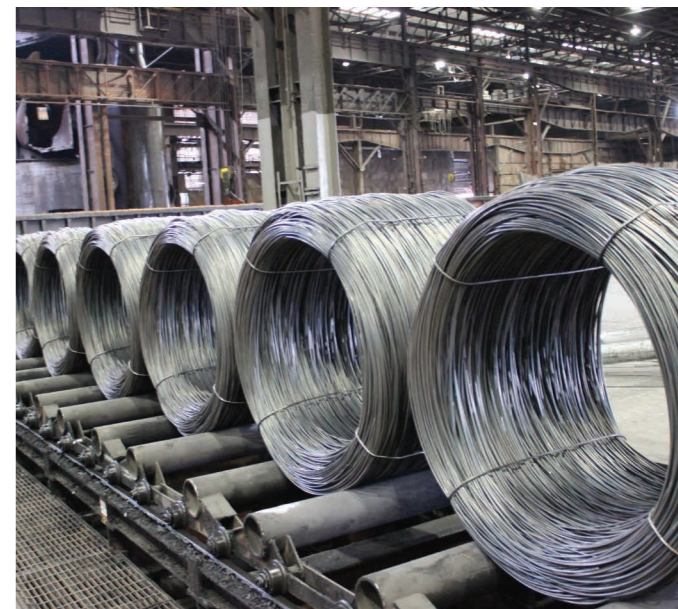
Compacted coils at unloading station
