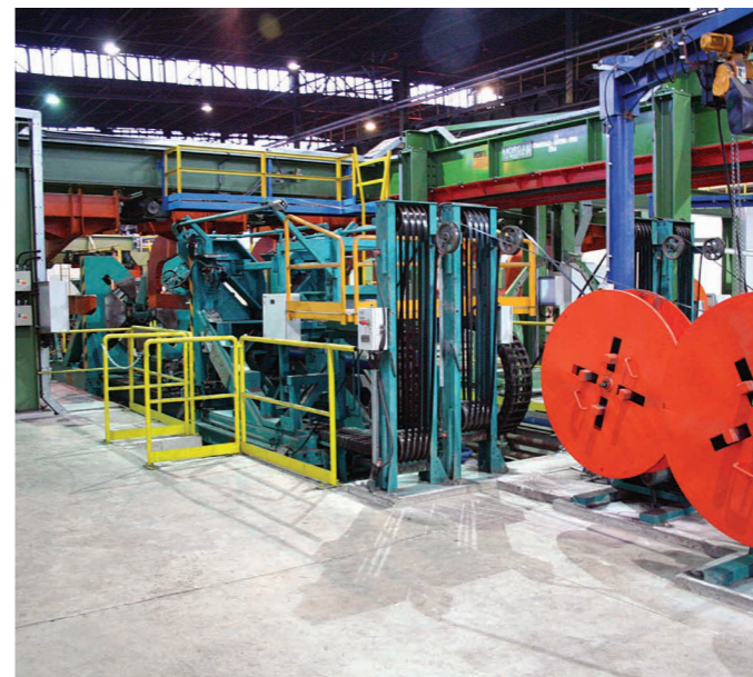
Horizontal compactor with strapping heads
