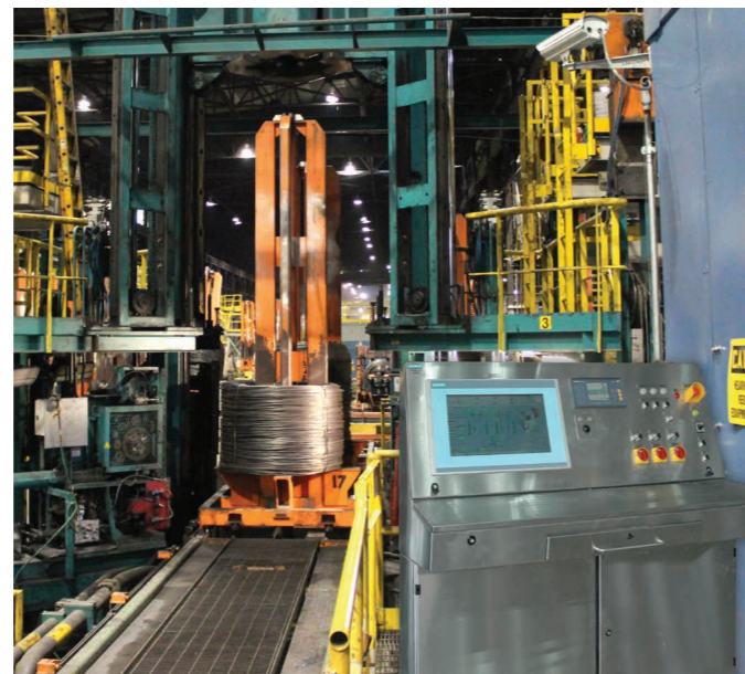
Compactor operator station
