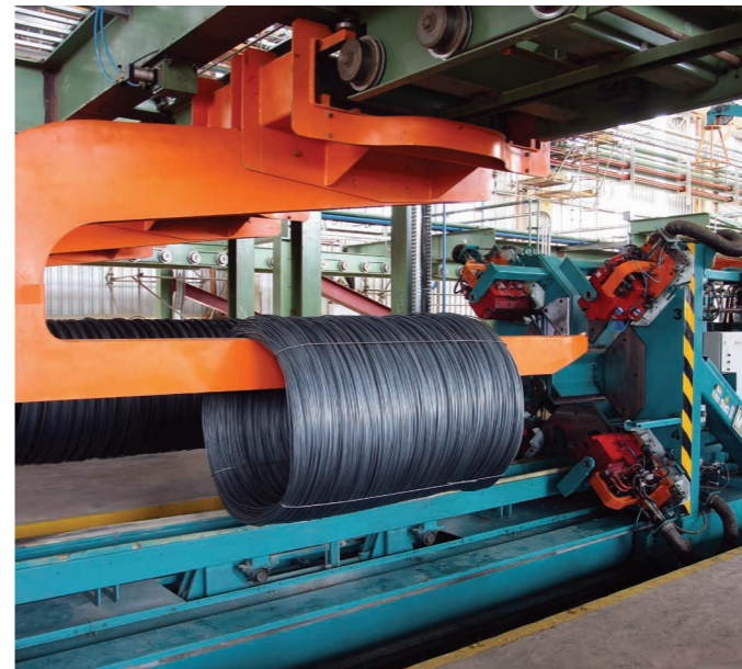
Compacted coil exiting horizontal compactor
